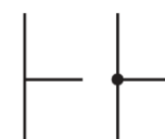
junction of conductors
