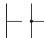
junction of conductors
